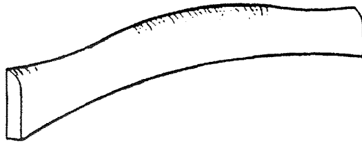
Type of jig required for shaping and moulding curved chair backs, etc.
